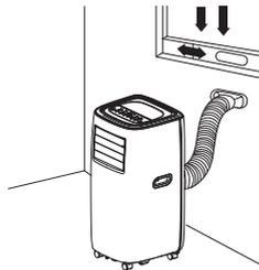
1. Partially open the window and place the extended slide bar in position before closing the window onto it.
